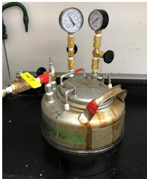
Figure 1 Pressure pot used to simulate water depth
